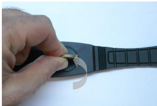
**Figure – Opening Battery Compartment**
